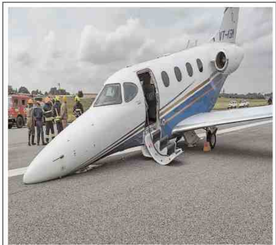
A private aircraft after it made an emergency landing due to a technical snag with its nose landing gear, at Hindustan Aeronautics Limited (HAL) airport in Bengaluru.
