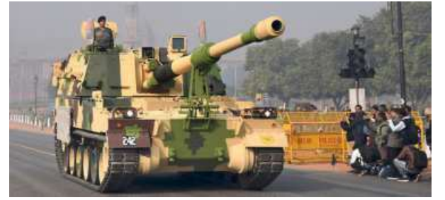
K-9 Vajra weighs 50 t and can fire shells up to 50 km SANDEEP SAXENA
